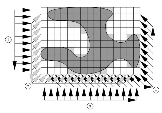
The scanner consists of four arrays of sensors arranged around a  $10 \times 15$  matrix. Array 1 consists of 10 sensors pointing to the right, array 2 has 24 sensors pointing diagonally to the top right, array 3 has 15 sensors pointing to the top and array 4 has 24 sensors pointing to the top left. Each sensor records the thickness of that portion of the object directly in front of that sensor.
